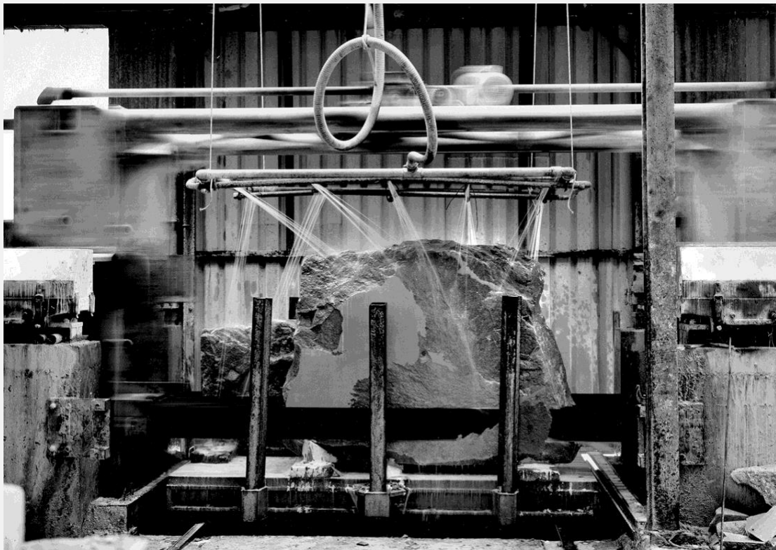
Purbeck-Portland Pond Free block on the frame saw. St Aldhelm's Quarry, 1992
